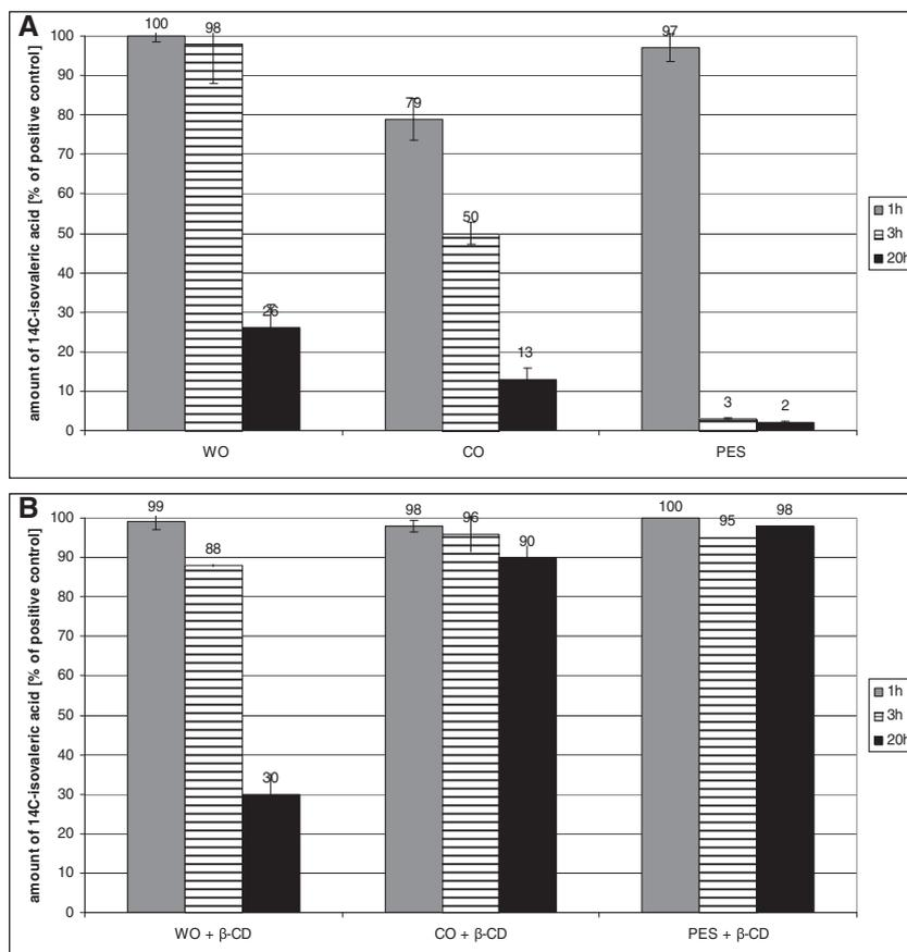
**Figure 2.** Scintigraphy of the recovery rate of WO, CO and PES samples after 1 h, 3 h and 20 h of incubation with  $^{14}\text{C}$ -isovaleric acid. (A) Untreated fabrics; (B) fabrics finished with  $\beta$ -cyclodextrin ( $\beta$ -CD). While the radioactive signal was almost completely present on WO samples after 3 h, it decreased over time on CO and rapidly on PES. The cyclodextrin finish significantly enhanced the retention of isovaleric acid on CO and PES
